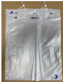
Diagram 1: Original PBAT/Talc/PLA Bag -Size: 25cm X 32cm -Holes from top: 5cm -Distance between holes: 10cm -Hole diameter:0.6cm
