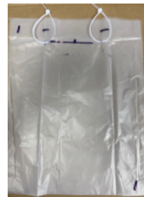
Diagram 4: Original PBAT/Talc/BPA-30 Bag -Size: 25cm X 32cm -Holes from top: 5cm -Distance between holes: 10cm -Hole diameter:0.6cm
