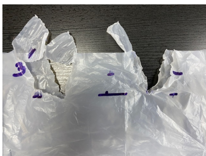
Diagram 3: Torn bag holder holes of the PBAT/Talc/PLA Bag.
